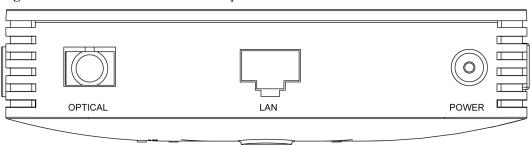
Figure 1-3 Ports and buttons on the rear panel of the HG8010
